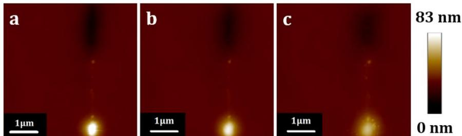
**Figure 3:** 2D AFM images of the PPF<sub>10°C</sub> after the scratching perturbation: (a) 90 s, (b) 327 s and (c) 2713 s.
