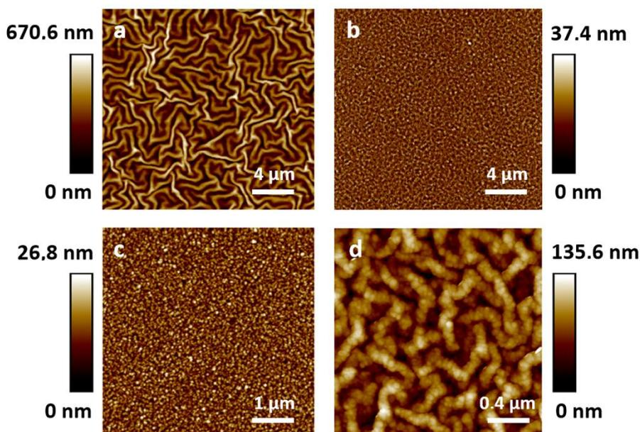
**Figure 8:** 2D AFM images of bilayer systems: (a) PPF<sub>10°C</sub> + Al; (b) PPF<sub>10°C</sub> annealed +Al; (c) PPF<sub>45°C</sub> + Al; (d) (PPF<sub>45°C</sub>)<sub>T=100°C</sub> +Al.
