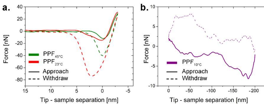
**Figure 1:** Typical force-distance curves recorded by AFM Peak Force measurements on (a) PPF<sub>45°C</sub>, PPF<sub>23°C</sub> and (b) PPF<sub>10°C</sub>.
