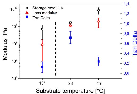
**Figure 2:** Evolution of the Tan Delta, storage and loss moduli of PPF as function of the substrate temperature. 10\* refers to a PPF<sub>10°C</sub> annealed for 1h at 150°C in air.
