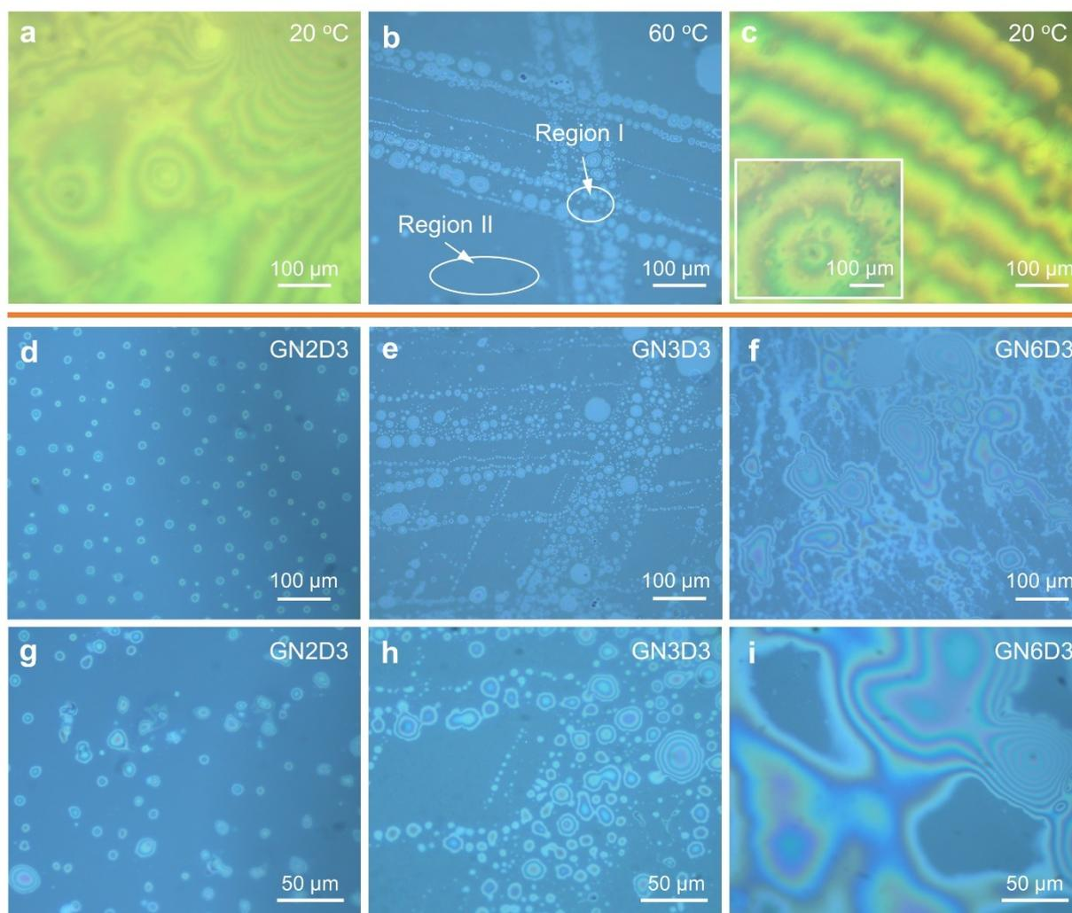
**Figure 4.** Visualization of microphase separation by fluorescent microscopy. **a–c**, Fluorescent images of thermoresponsive hydrogels (**a**) in the preparation state, (**b**) after immersing in water at 60 °C, and (**c**) after overnight recovery at room temperature using GN3D3 as a representative example. **d–i**, Fluorescence images of microphase-separated hydrogels of (**d,g**) GN2D3, (**e,h**) GN3D3 and (**f,i**) GN6D3 after immersing in water at 60 °C for 30 min.
