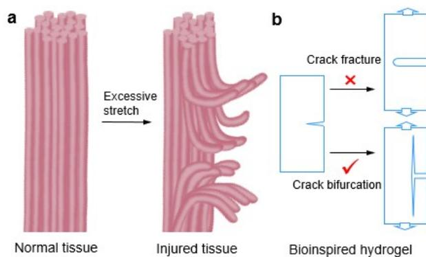
**Figure 1.** Biomimetic design of high-strength hydrogels. **a**, Simplified tearing model of fibrillar soft tissues<sup>5-8</sup> under excessive tension. **b**, Bioinspired design for crack-resistant hydrogels by deflecting the fracture along the stretching axis through crack bifurcation.
