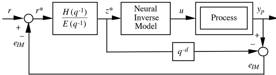
Fig. 9. An “internal model” control system to avoid.
