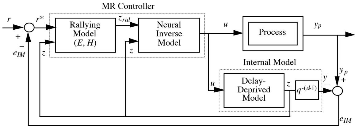
Fig. 5. The proposed internal model control system.
