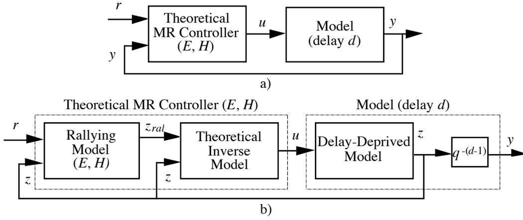
Fig. 2. The model reference controller equivalence.
