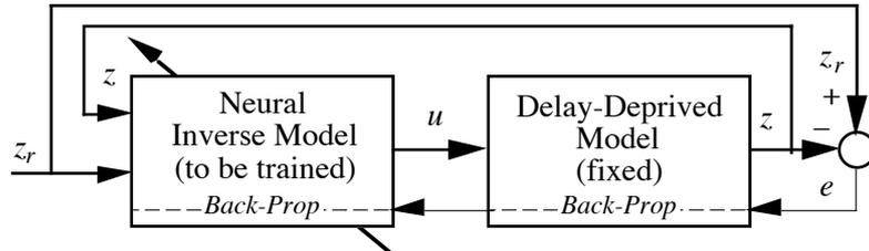
Fig. 3. The training system of the inverse model.
